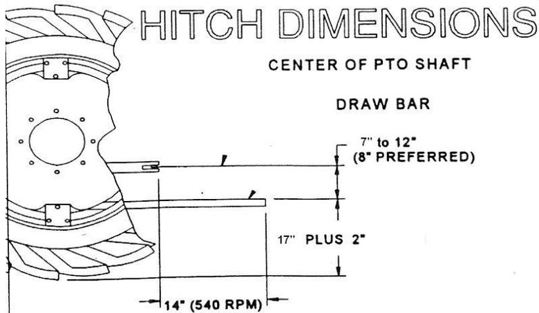
**Adjust the spreader hitch so the spreader is essentially level. Connect the safety chains to the tractor. Connect surge breakaway chain to tractor. Attach and secure, using approved hitch pin for load.**
