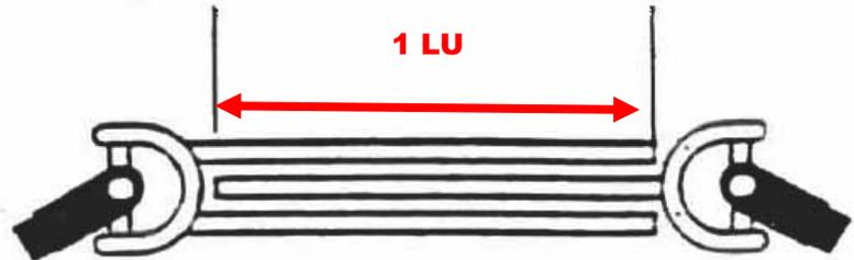
**To measure & trim the PTO:** Read and follow the instructions in the operator's manual from the PTO manufacturer. If the PTO is too long, **both** PTO Halves must be shortened by equal amounts.
