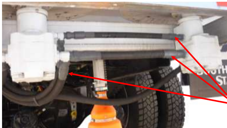
Case Drain and Pressure Line are completely sealed.
