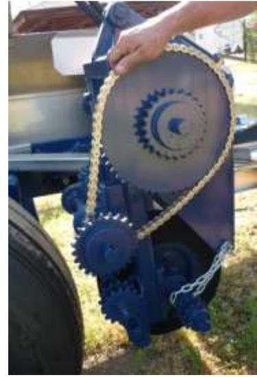
**3** Gently rotate sprocket until you can see the connecting link
