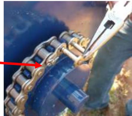
**5** Gripping with pliers remove plate, then remove prong. You can now remove the chain.
