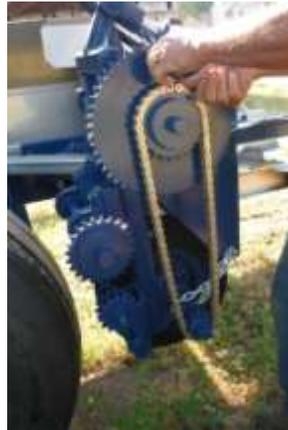
**2** Put chain on correct sprockets. Shown is the lime chain.
