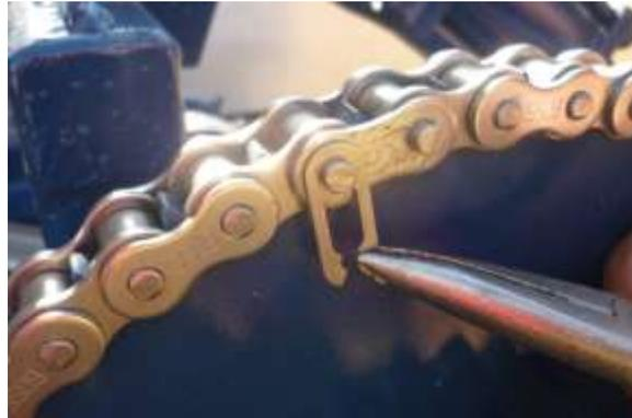
**4** Using needle nose pliers, pop the clip off the prong and carefully remove.
