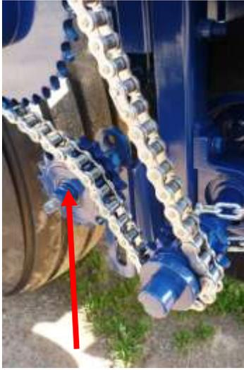
**1** Release the tension on the chain by moving the tension
