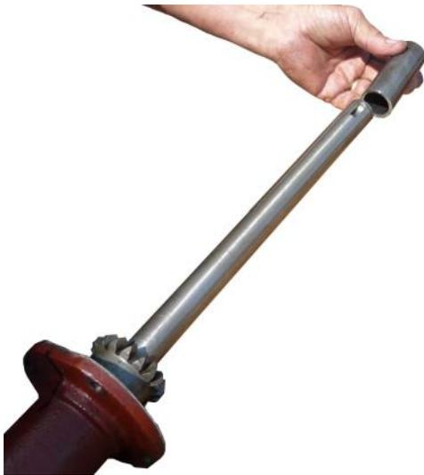
Slide GB-450338 Spacer, Pipe onto shaft and run shaft through GB-00125 Housing, Left & Right #13.
