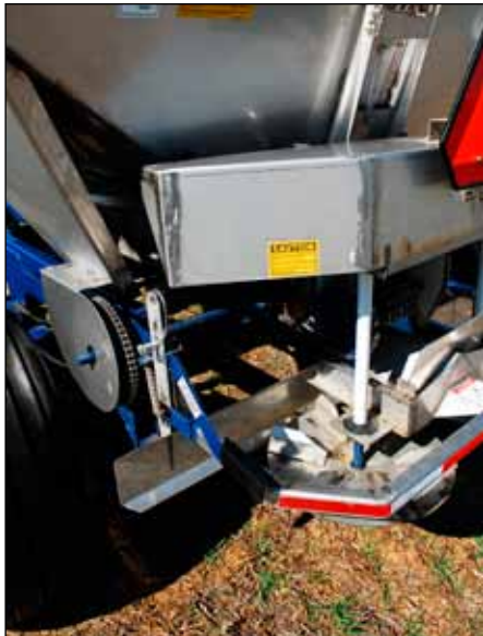
Positive Engagement Wheel Lock, Stainless Dishes, Less Parts
