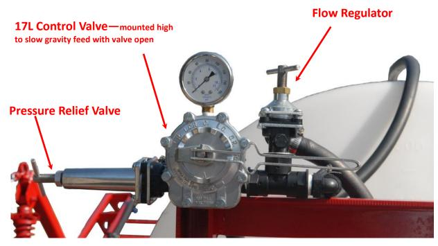
Pressure Relief Valve (PRV) moves in and out Move IN for Move OUT for **Control Valve (CV)** handle is straight out when ON. In the above photos the CV is in the OFF position.
