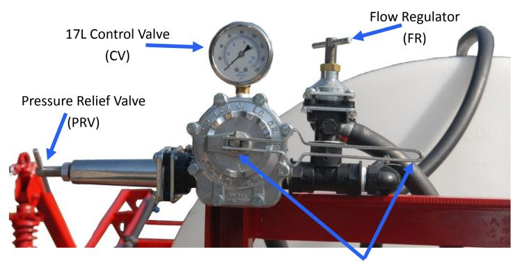
Control Valve in OFF position ON position— handle will be straight out
