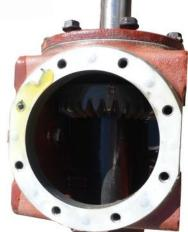
Assembled box shown. Bottom cap is underneath housing, shaft runs through center of housing, top cap sits on top of housing
