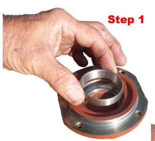
Drop GB-150102 Race into GB-051904 bottom cap. It should seat firmly.—may need to be tapped lightly with hammer.
