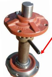
The GB-350009 roll pin will be hammered through the gear and shaft so that it
