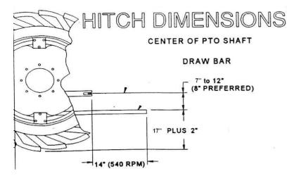
Adjust the spreader hitch so the spreader is essentially level. Connect the safety chains to the tractor. Connect surge breakaway chain to tractor. Attach and secure, using approved hitch pin for load.
