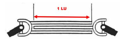
**To measure & trim the PTO**: Read and follow the instructions in the operator's manual from the PTO manufacturer. If the PTO is too long, **both** PTO Halves must be shortened by equal amounts.
