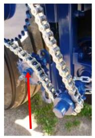
Release the tension on the chain by moving the tension
