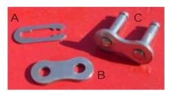
2 Connecting Link: Releases to move chains for different product and rates. A clip B plate C prong
