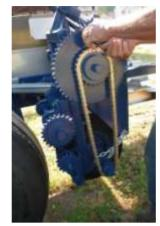
2 Put chain on correct sprockets. Shown is the lime chain.
