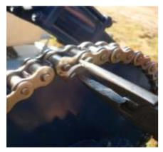
To make your chain proper length, a half length link may be required. A cotter pin secures the chain ends together
