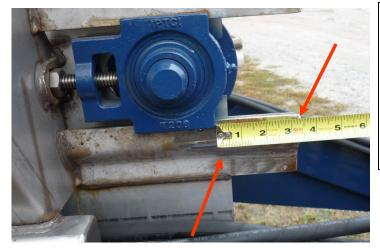
This measurement MUST be equal on both sides of the unit!
