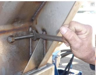
Step 1: Using a 1" wrench, loosen nut on take-up screw.
