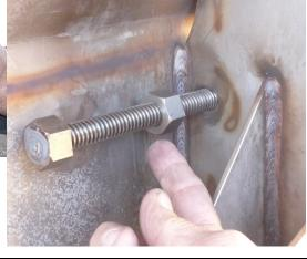
Step 2: Using a 1" socket will turn the screw to increase tension on front roller by moving it forward.
