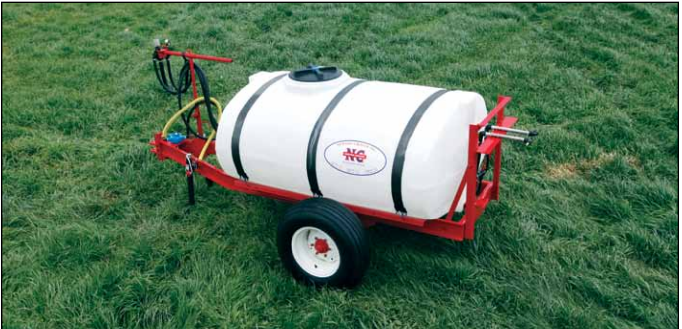
45 500 Gallon Nexus Sprayer with Hypro Roller Pump
