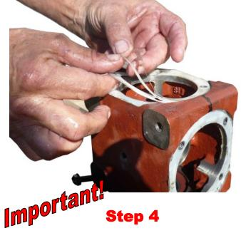
Be sure to count the spacers, type and number. You will need to replace these exactly when you reassemble your gear box.
