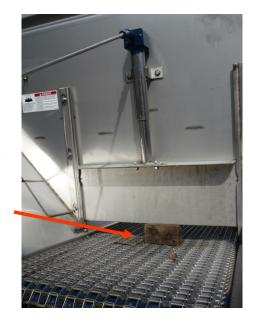
Step 9: Place a block of wood under gate to apply pressure to chain after it is draped onto rear roller
