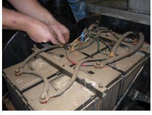
Completely remove wiring and battery connections
