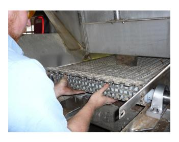
Step 10: Pulling chain under rear roller, remove as much slack as possible before cutting chain.
