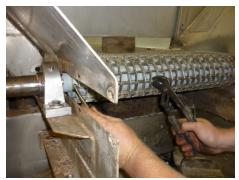
Step 13: Put nut on end of splice pin. Using pliers hold pin immobile and tighten nut using wrench.
