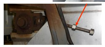
Step 2: Using wrench, remove the bolts from gate screw brace (1). Slide brace off end of handle.
