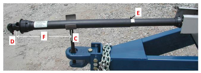
4 Separate PTO shaft and measure G (shaft overlap). NOTE: Measure from mark E to end of shaft (not shroud).
