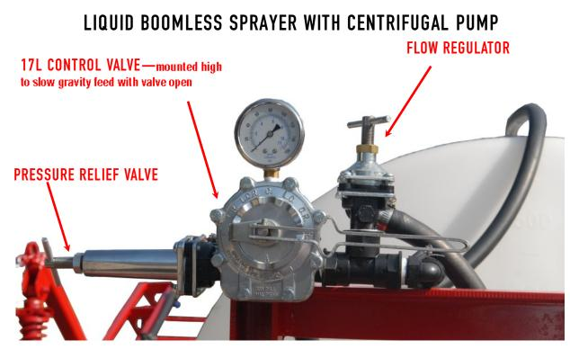
PRESSURE RELIEF VALVE (PRV) moves in and out
